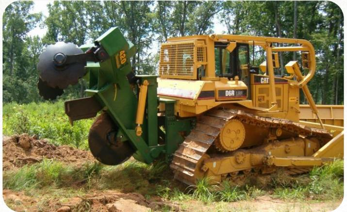
The Magnum 420 Mounted Sub-Soil Plow provides a high tilled 1.5m wide bed with an adjustable ripper designed for shallow 100% tillage or deep compacted soil sub-soiling. The disc configuration permits a better cutting action in debris and provides finer tillage, which assists in improved moisture and mineral retention, as well as herbaceous control. Runs on 180hp or greater dozers. “N” Model is a narrow version that cultivates 1.2m wide.
