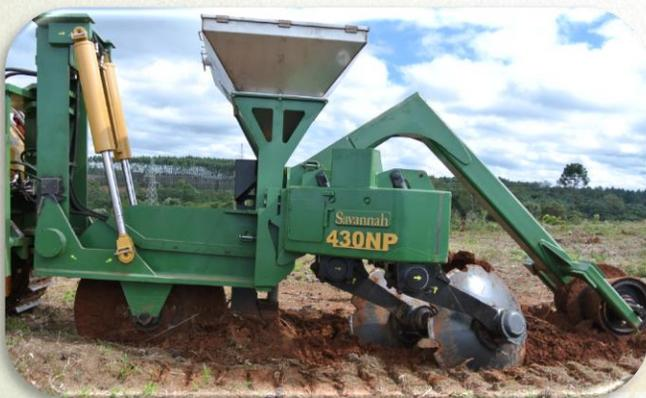
The lift assembly lifts into the rear of the dozer so the center of gravity moves towards the dozer. This essential feature extends the life of undercarriage components. The Stump-Jump™ Relieving Disc System allows discs to roll over stump residuals without forcing the plow from the ground, maximizing tillage quality and minimizing wear on the plow components.
