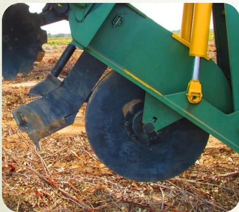
The abrasion resistant steel coulters mounted in front of the sub-tine eliminates chocking with roots and reduces pull force by 25%. The Savannah original ripper has hard changeable insert to ensure longer durability and easier maintenance
