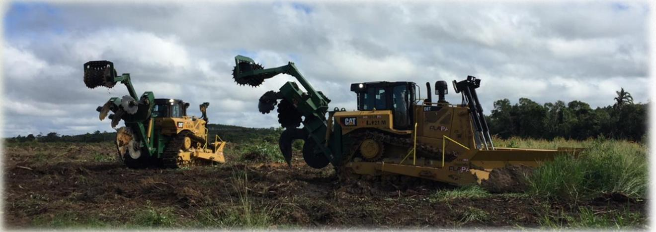
The Magnum 430N Mounted Sub-soil Plow has a “No Profile” tillage configuration. Discs are set with less pitch, allowing closer spacing, less drag, and greater cutting action. With less aggressive discs, fine tillage is achieved and provides a dense soil structure free of dirt clods and air pockets without an additional packer or chopper roller. The Magnum 430N has 1.6m working width.
