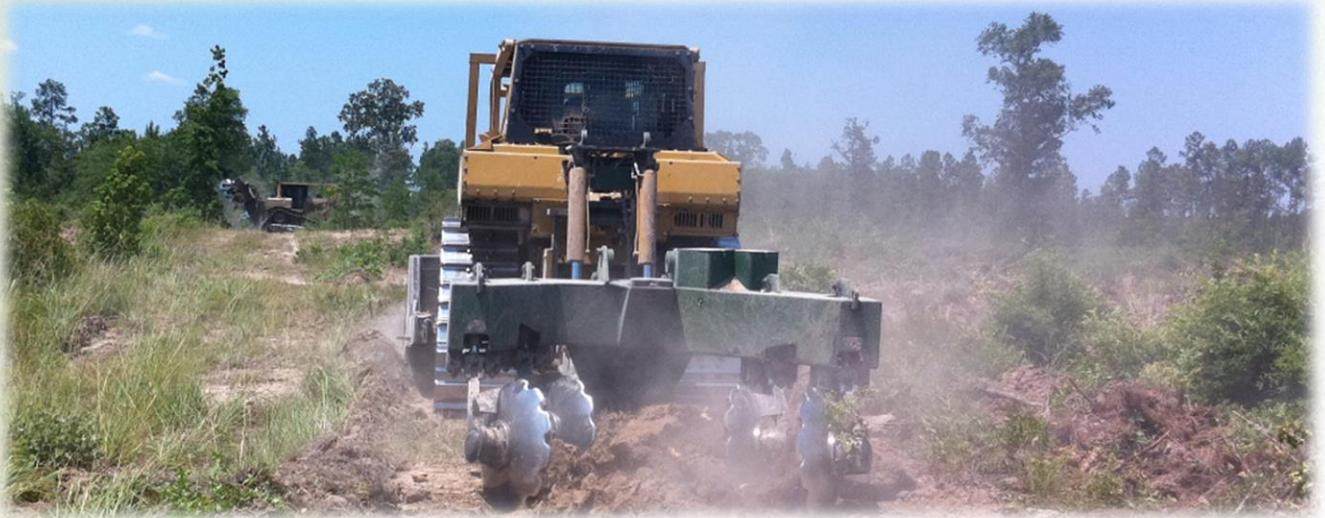
The Magnum 440 Mounted Sub-soil Plow provides a 2.3m wide well-defined bed over the rip-line. Runs on 250hp or greater dozers and, same as all the other Magnum 400 Plows, has mounts to add a packer or chopper roller to improve the compaction and density of heavy soils.
