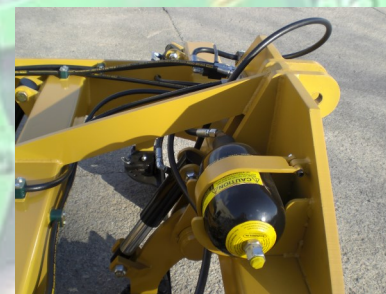
1 gal. accumulator relief system
