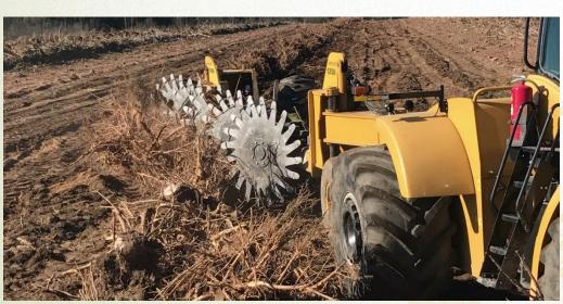
The Model 1720 Stump Puller and Savannah Rotary Rake equipment combination is the most productive method of converting planted forest to stump free conditions. When used together it is possible to convert from post harvest to windrowed stumps at a rate of 20-40 acres per day with 2 tractors, 1 stump puller and 1 Rotary Rake
